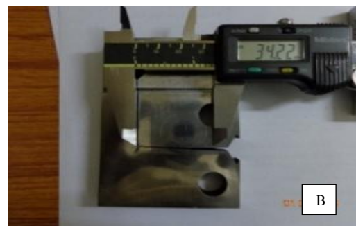
Fig. 2.2 (A.) Experimental setup of specimen with COD gauge during test; (B.) Measurement of final crack length by digital Vernier calipers.
